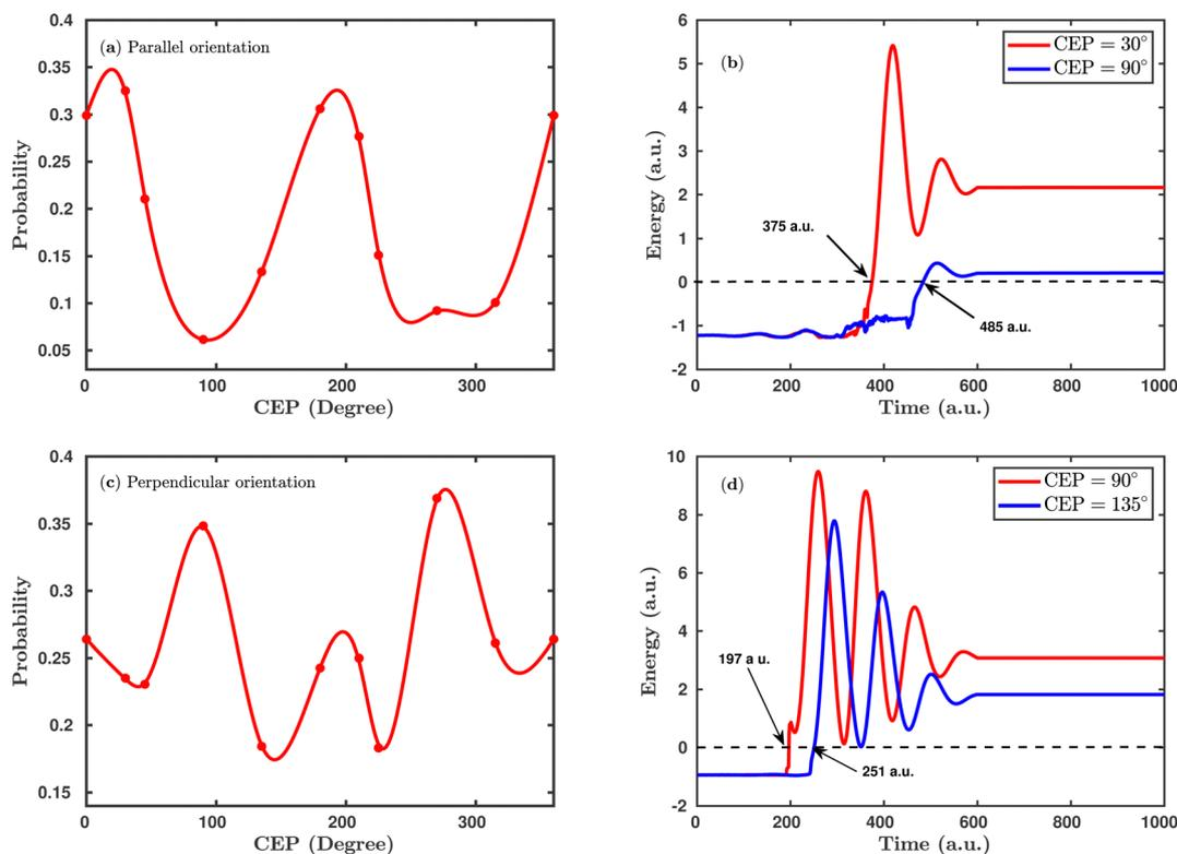
Fig. 4 (a) CEP-dependent single dissociative ionization channel probability in the case of parallel orientation. (b) The single particle energy of the ionized electron for CEP =  $30^\circ$  and CEP =  $90^\circ$  for the parallel orientation. (c) and (d) Same as (a) and (b), but for the perpendicular orientation. The arrows in (b) and (d) indicate the ionization time of the first ionization step. The peak intensity of the laser pulse is  $1 \times 10^{15} \text{ W cm}^{-2}$ .
