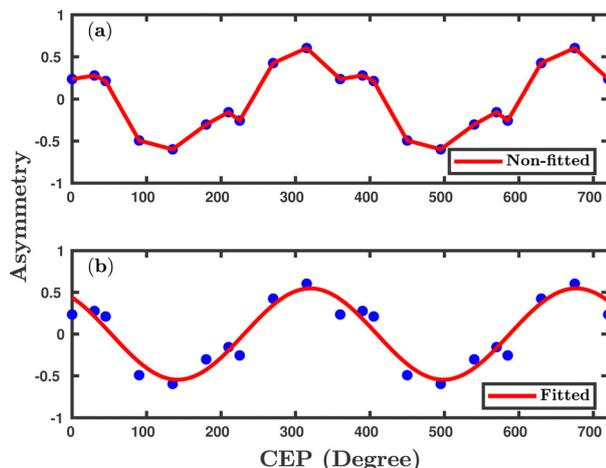
**Fig. 8** The asymmetry parameter to elucidate the effect of CEP. The initial orientation of the molecule is parallel to the laser polarization plane. The peak intensity of the laser pulse is  $1 \times 10^{15} \text{ W cm}^{-2}$ . (a) shows non-fitted data and (b) shows fitted data.
