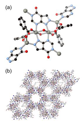
Fig. 9 (a) The coordination geometry of the L10 dianion in ALP-MOF 1 and 2 (zinc(II) and cobalt(II), respectively). (b) Extended structure of ALP-MOF 1 and 2 showing hexagonal channels capable of reversible and well-ordered water uptake. Zinc atoms coloured grey, cobalt atoms coloured dark blue.
