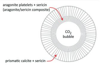
Fig. 5 Structure of the spherulite grown in the presence of sericin. Around the core cavity (a  $\rm CO_2$  bubble) aragonite and calcite grow in concentric shells. Modified from Pastero and Aquilano.<sup>34</sup>
