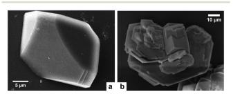
**Fig. 2** Calcium carbonate polymorph grown in the presence of lithium in solution: (a) calcite cleavage rhombohedron with initial rounding of corners and apexes (modified from Aquilano et al. <sup>46</sup>); (b) prismatic aragonite crystals associated with flat, pseudo-hexagonal calcite crystals (modified from Aquilano et al. <sup>16</sup>).
