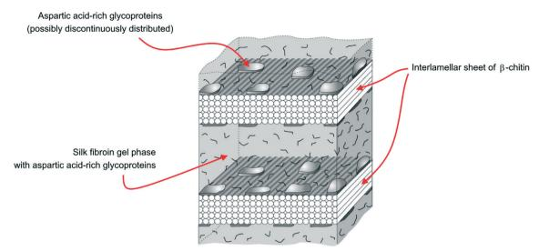
Fig. 4 The demineralized layer of the organic scaffold in the *Atrina* shell, showing the interlamellar sheet of β-chitin pinched between two layers of silk fibroin gel (modified from Levi-Kalisman et al.<sup>59</sup>).
