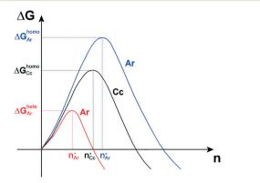
Fig. 6 Qualitative activation energies ( $\Delta G_{Ar}^{hete}$  and  $\Delta G_{Ar}^{homo}$ ) and critical nuclei  $(n_{Ar}^*)$  for heterogeneous (red line) and homogeneous (blue line) nucleation of aragonite, Ar, in supersaturated aqueous solutions. The activation energy and critical nucleus for homogeneous nucleation (black line) of calcite, Cc, are also reported ( $\Delta G_{Cc}^{homo}$  and  $n_{Cc}^*$ ).
