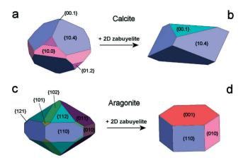
**Fig. 3** Equilibrium shapes of calcite and aragonite at 0 K. Calcite (a) and aragonite (c) in the vacuum; calcite (b) and aragonite (d), after the 2D-epitaxial adsorption of zabuyelite above  $(00.1)_{Cc}$ ,  $(10.4)_{Cc}$  and  $(001)_{Ar}$ . Redrawn from Aquilano et al. <sup>46</sup>
