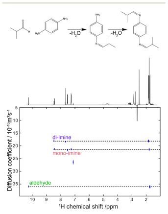
Fig. 10 DOSY spectrum obtained during a di-imination reaction monitored by online NMR at a flow rate of 3 mL min<sup>-1</sup>. The experiment duration was 80 s. Adapted with permission from ref. 199. © 2022 Wiley-VCH GmbH.
