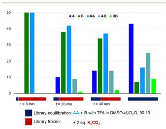
Fig. 4 The equilibration of a library starting from AA (14 mM) and B (14 mM) with TFA (14 mM) in DMSO-d<sub>6</sub>/D<sub>2</sub>O (90:10) can be brought to a halt by the addition of  $K_2CO_3$  (28 mM). The libraries were analysed by <sup>1</sup>H NMR spectroscopy after 5 hours, independent of the moment at which the library was frozen, and the results are shown in mol%
