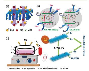
Fig. 10 Schematic illustration of (a) rejection and (b) photocatalytic degradation of dye molecules over the NH2-MIL-101(Fe) and MIL-101(Fe) MOF-integrated membranes and (c) pictorial illustration of degradation setup and its mechanism. Reproduced from ref. 139 with permission from Elsevier Inc, copyright 2022.
