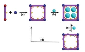
Fig. 3 A regenerative MOF for reversible uptake of Cd(II): (a) self assembly 3D framework from organic ligand and hard metal ion; (b) effective absorption with high capacity; (c) absorption and desorption; (d) reconstruction of the used sample into a fresh sample. Reproduced from ref. 96 with permission from Royal Society of Chemistry, copyright 2016.
