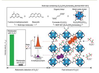
Fig. 5 Schematic of the ratiometric detection and simultaneous removal of Cr<sub>2</sub>O<sub>7</sub><sup>2-</sup> using multi-dye (resorufin and 7-amino-4-methylcoumarin) containing MOF-801. Reproduced from ref. 115 with permission from Elsevier Inc, copyright 2019.
