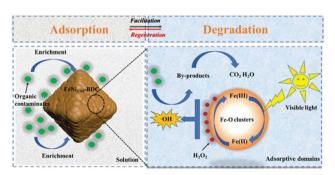
Fig. 8 Schematic illustration of contaminant removal in FeNi<sub>1/60</sub>-BDC/ H<sub>2</sub>O<sub>2</sub>/visible light system. Reproduced from ref. 136 with permission from Elsevier Inc, copyright 2021.
