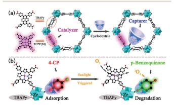
Fig. 15 (a) The construction of CMCD@NU-1000-TCPP(Pd) and (b) schematic illustration of the adsorption and degradation processes toward 4-CP. Reproduced from ref. 170 with permission from American Chemical Society, copyright 2021.
