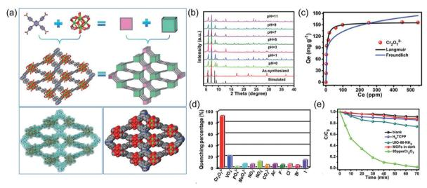
Fig. 6 (a) The structure illustration of JLU-MOF60; (b) the stability of JLU-MOF60 in various pHs; (c) the removal ability; (d) the sensing ability and (e) the degradation ability of JLU-MOF60 for  $Cr_2O_7^{2-}$  treatment. Reproduced from ref. 122 with permission from Royal Society of Chemistry, copyright 2019.
