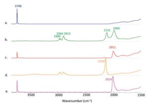
Fig. 1 Diffuse reflectance infrared Fourier transform spectra of SBA-15<sub>700</sub> (a),  $\equiv$  SiOAl(Cp\*IrH<sub>3</sub>)<sub>2</sub> **2-s** (b), **Ir-Al/SiO<sub>2</sub>** (c), Cp\*IrH<sub>4</sub> physisorbed on SBA-15<sub>700</sub> (d) and Ir/SiO<sub>2</sub> (e) recorded on powder materials under argon.
