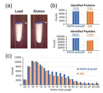
Fig. 2 AnExSP for polyacrylamide gel-extracted proteins containing CBB. (a) AX SPE disc: after loading a CBB-containing HCPE (Load) and after peptide elution (Elution). White arrows: Trapped CBB. (b and c) Comparison between PEPPI-AnExSP and IGD: identified proteins/peptides (b) and amino acid lengths of identified peptides (c).
