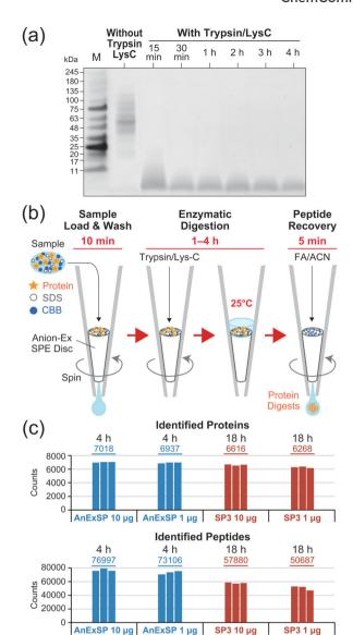
Fig. 1 Sample pretreatment for bottom-up MS using AnExSP. (a) SDS-PAGE of digested HCPE recovered from AX SPE discs. After digestion of HCPE with Trypsin/Lys-C, digestion products recovered from AX SPE discs with 10% SDS were separated by SDS-PAGE and visualized with CBB. The substrate enzyme ratio was set to 20:1. M: molecular weight marker. (b) Schematic workflow of AnExSP. FA: formic acid. ACN: acetonitrile (c) DIA analysis of digestion products.
