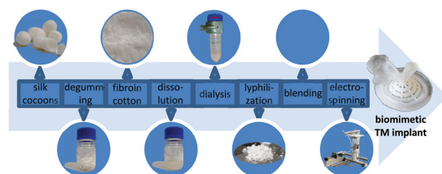
Fig. 1 Schematic workflow from Bombyx mori silkworm cocoon to a TM implant with morphologically biomimetic, mechanical and oscillatory properties.
