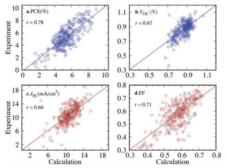
Fig. 9 ML-predicted versus experimental data for PCE,  $V_{\rm OC}$ ,  $J_{\rm SC}$ , and FF for all data points (300 OPVs) using the leave-one-out cross validation approach. Reprinted with permission from ref. 435. Copyright 2021 American Chemical Society.
