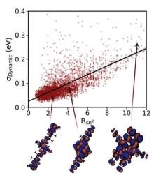
Fig. 7 Correlation between dynamic disorder  $\sigma_{Dvnamic}$  and fraction of sp<sup>2</sup> atoms in contact (expressed in percentage) in molecular crystals: head to tail arrangement is surprisingly favourable for charge transport.
