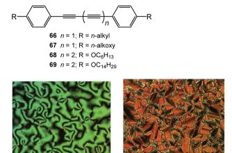
Structures of **66–69**. Polarised-light optical microscopy images of 69 at 130 °C (left) and 117 °C (right). Reproduced from ref. 183 with permission from the Royal Society of Chemistry
