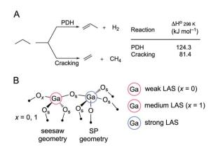
Scheme 1 (A) Competing propane dehydrogenation (PDH) and propane cracking reactions. (B) A possible coordination geometry for a  $Ga_{IV}$ –O– $Ga_{VI}$  surface linkage with the attribution of Lewis acidity strength according to the  $^{15}N$  chemical shift of bound pyridine probe molecule. $^{12}$  SP stands for square pyramidal.
