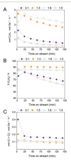
**Fig. 3** Results of the PDH catalytic tests, *i.e.* Ga weight-normalized activity (A), selectivity to propene (B), and formation rates to cracking products (combined rates to ethene and methane), (C) for the  $(Ga,Al)_2O_3$  catalysts. WHSV = 7.2 h $^{-1}$ , T=550 °C. Initial and final conversions and selectivities are presented in Table S5,† while surface area-normalized, Ga-weight normalized activities and productivities are in Table S6.†
