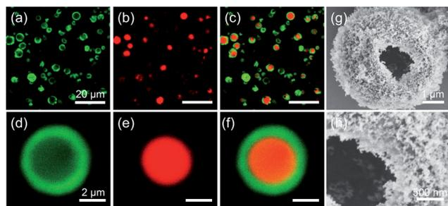
Fig. 2 (a)–(f) CLSM images of M-HPMs at different magnifications: (a) and (d) the zein was labelled by FITC under a green channel, (b) and (e) the oil was stained by Nile red under a red channel and (c) and (f) the overlays of two stained images. (g) and (h) SEM images of broken M-HPMs. Scale bars are (a)–(c) 20 μm, (d)–(f) 2 μm.
