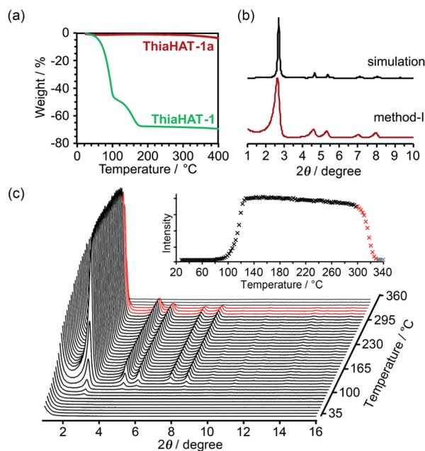
Fig. 6 (a) TG profiles of ThiaHAT-1 (green line) and ThiaHAT-1a (red line). (b) PXRD pattern of ThiaHAT-1a activated *via* method I with the simulation pattern of ThiaHAT-1. (c) VT-PXRD patterns of ThiaHAT-1 heated from RT to 360 °C. Inset: changes of the (100) peak intensity of ThiaHAT-1 with temperature. The intensity rapidly decreased from 305 °C (red line), which indicated the collapse of the framework and no peak was detected at over 330 °C.
