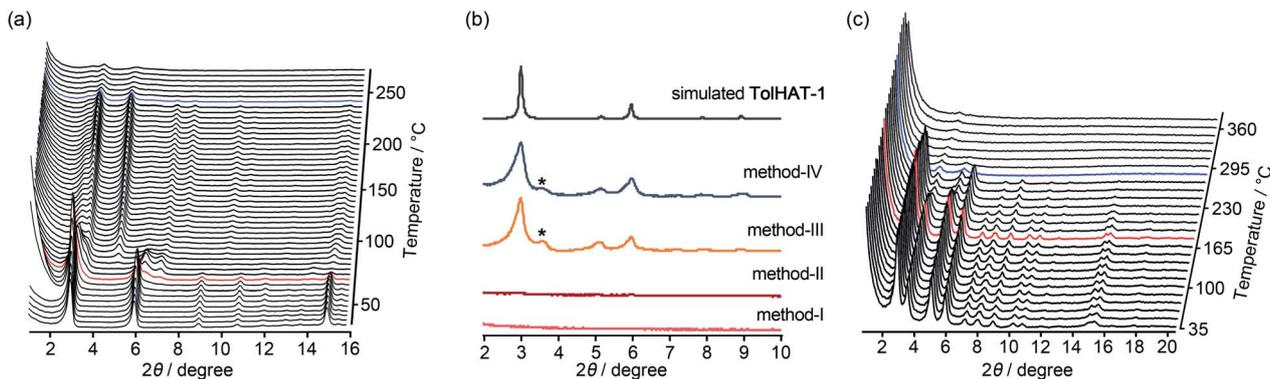
Fig. 5 (a) Variable temperature (VT)-PXRD patterns of the as-formed HOF TolHAT-1. (b) PXRD patterns of activated HOF TolHAT-1aN ( $N = I-IV$ ) with the simulation pattern of TolHAT-1. (c) VT-PXRD patterns of TolHAT-1aIV from rt to 360 °C. Red line indicates the temperature where the network begins to collapse and blue line corresponds to the temperature where the framework is fully collapsed. The asterisk (\*) denotes a non-identifiable peak appeared for the activated TolHAT samples.
