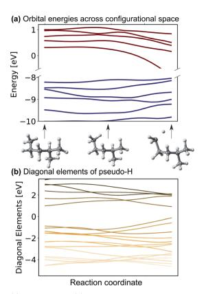
Fig. 2 (a) Eigenvalues and (b) diagonal matrix elements of the pseudo-Hamiltonian of the SchNet + H model trained on molecules of the QM7-X data set  $^{52}$  along a trajectory of conformational change in 2-methylpentane.
