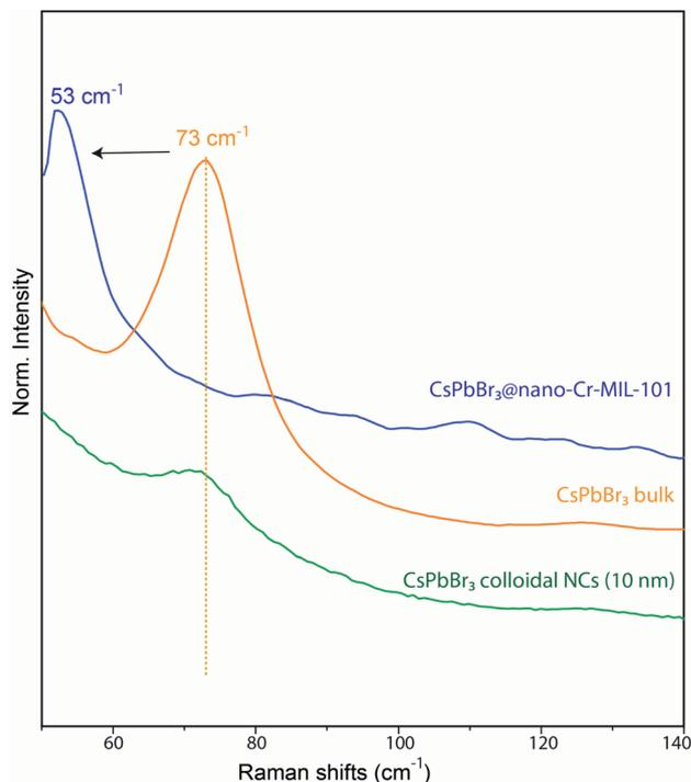
Fig. 3 Comparison between Raman vibrational bands of bulk CsPbBr<sub>3</sub>, CsPbBr<sub>3</sub>@nano-Cr-MIL-101, and colloidal CsPbBr<sub>3</sub> NCs (10 nm).
