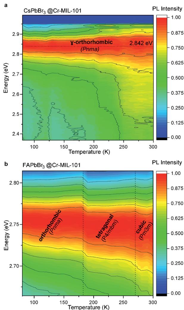
Fig. 5 (a) Photoluminescence evolution over temperature (from 80 to 300 K) for CsPbBr<sub>3</sub>@nano-Cr-MIL-101. (b) Photoluminescence evolution over temperature (from 80 to 300 K) for FAPbBr<sub>3</sub>@nano-Cr-MIL-101.
