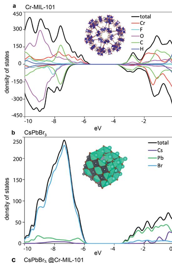
Fig. 6 Electronic density of states calculated for (a) Cr-MIL-101 and (b) nano CsPbBr<sub>3</sub>. (c) Minimum-energy geometry for CsPbBr<sub>3</sub>@nano-Cr-MIL-101.
