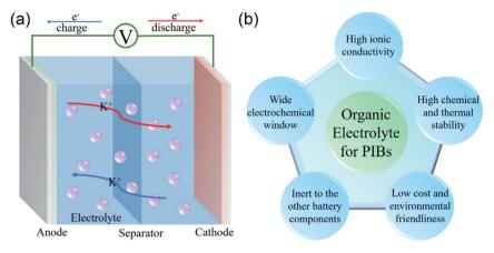
Fig. 1 (a) Schematic operation principle of PIBs. (b) The requirements of organic electrolytes for PIBs.
