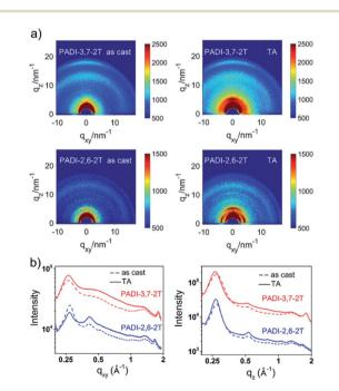
Fig. 5 (a) GIXD patterns of PADI-3,7-2T and PADI-2,6-2T thin films (as cast and thermal annealing (TA) at 70 °C); (b) line-cut profiles of inplane and out-of-plane.
