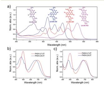
Fig. 4 UV-Vis absorption spectra of (a) monomers in toluene solution, and (b) PADI-3,7-2T and (c) PADI-2,6-2T in toluene  $(10^{-5} \text{ M})$  and in film.
