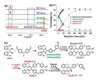
Fig. 2 (a) Monitoring the polymerization using (S,S)-1 and 2a by *in situ*  $^1$ H NMR spectroscopy in DMF- $d_7$ . (b) Plots showing consumption of 2a (black), formation of the imidazolidine intermediate (green), and phenolic O–H groups (blue and red). (c) Detailed polymerization mechanism.
