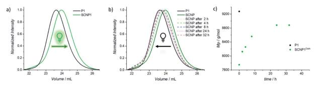
Fig. 1 (a) Normalized UV-SEC-trace at 250 nm of the crosslinker mediated folding of P1 (black line) with BisTAD using green light ( $\lambda_{max} = 525$  nm). The resulting collapsed polymer chain is displayed in dark green (SCNP1). (b) Normalized UV-SEC-traces at 250 nm of the stepwise unfolding process of SCNP1 over time in the dark. (c) Evolution of  $M_P$  during the stepwise unfolding process over time of SCNP1.
