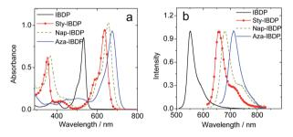
Fig. 1 (a) UV-vis absorption spectra of the compounds. (b) Normalized fluorescence spectra of the compounds.  $c=1.0\times10^{-5}$  M in 2-methyltetrahydrofuran, 20 °C.
