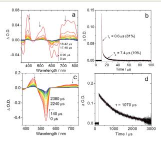
Fig. 3 Nanosecond time-resolved transient absorption spectra of the compounds in frozen solution at 77 K. (a) Sty-IBDP upon nanosecond pulsed laser excitation ( $\lambda_{ex} = 600$  nm) and (b) decay trace of Sty-IBDP at 390 nm. (c) IBDP upon ns pulsed laser excitation ( $\lambda_{ex} = 533$  nm) and (d) decay trace of IBDP at 450 nm.  $c = 1.0 \times 10^{-5}$  M in deaerated 2methyltetrahydrofuran at 77 K
