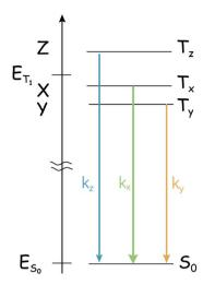
Scheme 1 Typical energy diagram for a triplet state  $(T_1)$ , showing the lifting of the degeneracy of the sublevels in the case of an orthorhombic D-tensor. The ground state  $S_0$  is also presented.  $E_{T_1} - E_{S_0}$  is in the order of  $10^4$  cm<sup>-1</sup>, whereas |Z - X| is in the order of fractions of cm<sup>-1</sup>. The scheme represents the case of the ZFS parameter D < 0.
