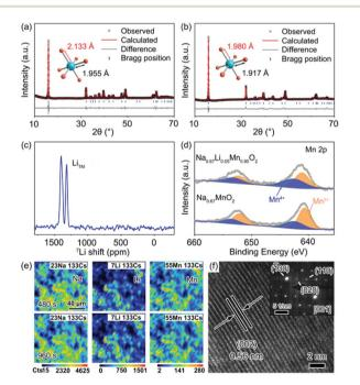
Fig. 1 Rietveld refinement of powder XRD patterns for (a) P'2- $Na_{0.67}MnO_2$  and (b) P'2-Na<sub>0.67</sub>Li<sub>0.05</sub>Mn<sub>0.95</sub>O<sub>2</sub>. (c) <sup>7</sup>Li ss-NMR of P'2-Na<sub>0.67</sub>Li<sub>0.05</sub>Mn<sub>0.95</sub>O<sub>2</sub>. (d) XPS spectra of the Mn 2p region of  $Na_{0.67}MnO_2 \quad and \quad P'2-Na_{0.67}Li_{0.05}Mn_{0.95}O_2.$ (e) Elemental SIMS mappings and (f) HRTEM and SAED images  $Na_{0.67}Li_{0.05}Mn_{0.95}O_2$
