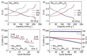
Fig. 6 Charge and discharge profiles of (a) P'2-Na $_{0.67}$ MnO $_2$  and (b) P'2-Na $_{0.67}$ Li $_{0.05}$ Mn $_{0.95}$ O $_2$  at 20 mA g $^{-1}$ . (c) Rate capability comparison of and P'2-Na $_{0.67}$ MnO $_2$  and P'2-Na $_{0.67}$ Li $_{0.05}$ Mn $_{0.95}$ O $_2$  at different rates. (d) Cycle performance of P'2-Na $_{0.67}$ MnO $_2$  and P'2-Na $_{0.67}$ Li $_{0.05}$ -Mn $_{0.95}$ O $_2$  at 50 mA g $^{-1}$ .
