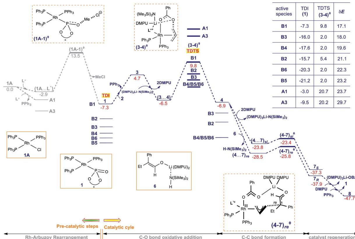
Fig. 4 The overall Gibbs free energy profile (kcal mol<sup>–1</sup>) for the Rh-catalyzed asymmetric allylic alkylation of 2-phenylbutanal by allyl benzoate. The activation span (ΔE) for different likely active catalysts is tabulated for comparison.
