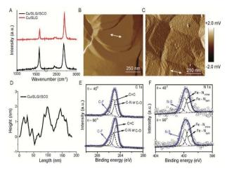
Fig. 2 (A) Raman spectra of SLG before (red) and after adsorption (black) of  $[Fe^{III}(qsal-I)_2]NTf_2$ . AFM amplitude images of (B) bare graphene and (C) after adsorption of  $[Fe^{III}(qsal-I)_2]NTf_2$  and the corresponding AFM height profiles (D). Angle dependent X-ray photoelectron spectra of (E) C 1s, and (F) N 1s (see section S1 for all other spectra).
