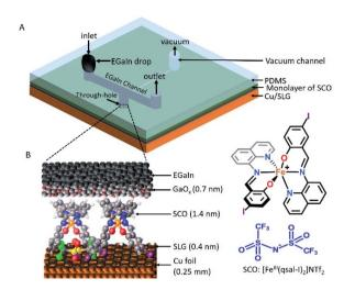
Fig. 1 (A) Schematic illustration of the SCO molecule based device with the EGaIn top-electrode stabilized in a small through-hole in a rubber stamp (made of PDMS) and (B) the SCO based molecular junction of the form of Cu//SLG//[Fe<sup>III</sup>(qsal-I)<sub>2</sub>]NTf<sub>2</sub>//GaO<sub>x</sub>/EGaIn (EGaIn = eutectic alloy of Ga and In).
