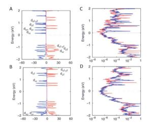
Fig. 6 Projected density of states (PDOS) of  $[Fe(qsal-I)_2]NTf_2$  for the high spin state (A) and low spin state (B). The projected transmission spectrum of  $[Fe(qsal-I)_2]NTf_2$  for the high spin state (C) and low spin state (D). Red and blue colors stand for alpha and beta spin–orbitals. The filled curves are the PDOS of the Fe<sup>III</sup> metal.
