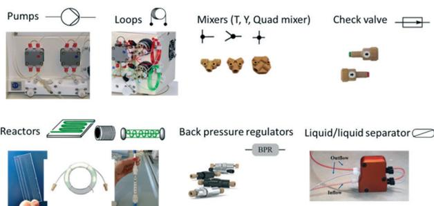
Fig. 2 Flow equipment and representation.
