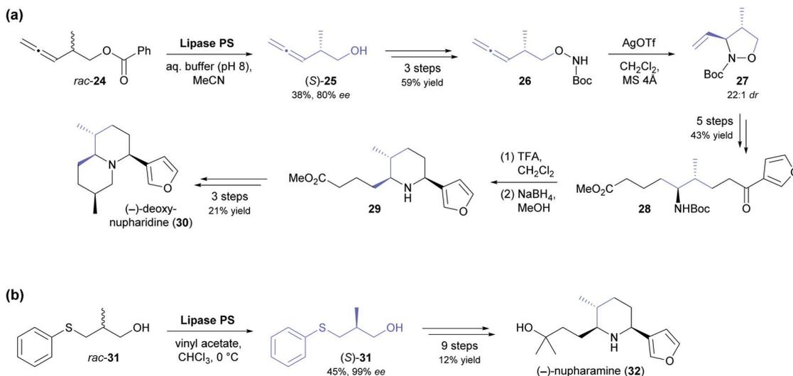
**Scheme 4** Lipase-catalysed kinetic resolution of  $\beta$ -chiral primary alcohols in the asymmetric synthesis of Nuphar alkaloids: (a) chemo-enzymatic synthesis of (-)-deoxynupharidine (30), (b) chemo-enzymatic synthesis of (-)-nupharamine (32).
