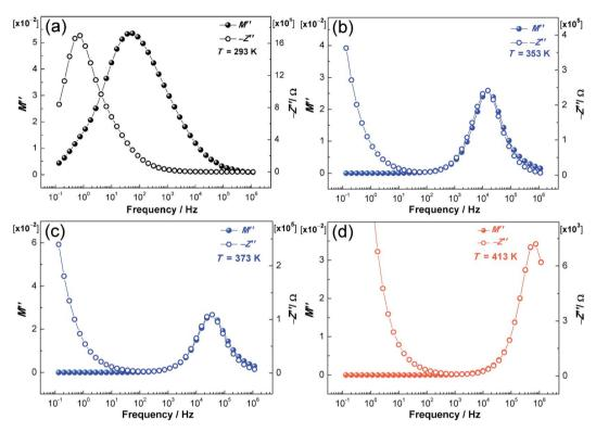
Fig. 7 The temperature dependence of M'' (the imaginary part of complex electric modulus) and -Z'' (the imaginary part of the complex impedance) at selected temperatures of 293 K (a), 353 K (b), 373 K (c) and 413 K (d).
