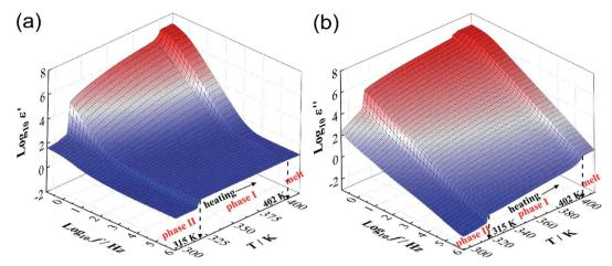
Fig. 2 The temperature and frequency dependence of (a)  $\varepsilon'$  and (b)  $\varepsilon''$ . Both graphs clearly show the two jumps at 315 K and 402 K during the heating process, respectively.
