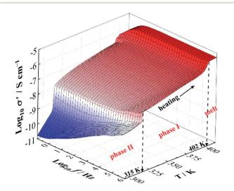
Fig. 3 Three dimensional (3D) graph of the real part of complex conductivity ( $\sigma'$ ) as a function of frequency ( $10^{-1}$  to  $10^{6}$  Hz) and temperature (between 293 K and 413 K).
