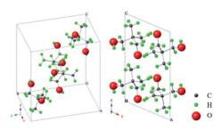
Scheme 1 Crystal structure (monoclinic phase) of NPG at 295 K.<sup>15</sup> Notes: left, view along (1 1 1) crystal plane; right, view along (0 1 0) crystal plane.
