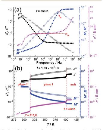
Fig. 1 (a) The frequency-dependent dielectric properties of NPG recorded at 353 K (in the plastic crystalline state) in the frequency range of  $10^{-1}$  to  $10^6$  Hz and (b) the temperature-dependent dielectric properties of NPG at 133 Hz in the temperature range of 293-413 K. Note: dielectric properties are shown in three representations: the complex permittivity ( $\varepsilon^*$ ), the complex conductivity ( $\sigma^*$ ) and the complex electric modulus (M\*).
