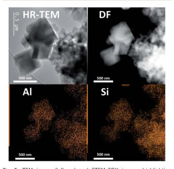
Fig. 5 TEM image (left up) and STEM-EDX images highlighting homogenous Si and Al distribution encountered in Al-densified (amorphous) equilibrium compositions collected after 45 min from the synthesis system in ref. 65 (Si/Al $_{\rm S}=3$ , see Fig. 4).
