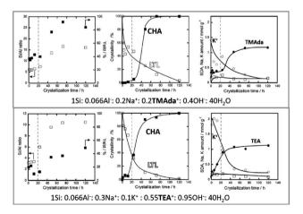
Fig. 6 Evolution of LTL-to-CHA partial IZC (Si/Al $_{\rm P}=3.0$ ; Si/Al $_{\rm B}=15$ ), adapted from Nishitoba *et al.*<sup>107</sup> A period with stable compositions is discerned prior to nucleation and growth (dotted line). The molar compositions do not account for the high K-content in the parent phase (16%  $\rm K_2O$ ).
