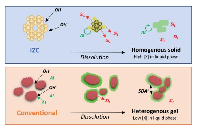
Fig. 7 Physical states and Al concentrations (red = siliceous, green = aluminous) through the stages of dissolution starting from high Si/Al<sub>P</sub> materials. Relatively homogeneous distributions of Al (no gradients) are found within the remnant solid after IZC dissolution as opposed to the conventional case yielding a heterogeneous gel.
