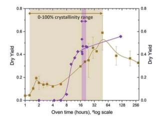
Fig. 11 Temporal evolution of alkali-free ZSM-5 (MFI; Si/Al = 40) synthesis from amorphous sources (purple) and IZC (brown): dry yields (y-axis) and crystallinity ranges. The filled background represents the assembly stage (III) for each. Based on supporting info in ref. 47.
