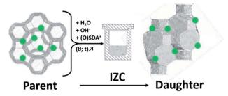
**Fig. 1** Schematic representation of interzeolite conversion (IZC) from a parent zeolite and some additional reagents ( $H_2O$ ,  $OH^-$  and some SDA). Crystallization of a daughter zeolite occurs at elevated temperature ( $\theta$ ) and prolonged exposure time (t). Green dots indicate framework Al positions.
