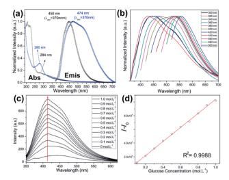
Fig. 2 (a) Absorption (Abs) and emission (Emis) spectra acquired at room temperature of C-dot-NH<sub>2</sub> (black) and PBAC-dots (blue); (b) normalized emission spectra as function of excitation wavelength of PBAC-dots; (c) emission spectra as function of glucose concentration of PBAC-dots; (d) linear plot of integrated emission as function of glucose concentration. *I*<sub>0</sub> and *I* are the integrated emission spectra of PBAC-dots in absence and presence of the analyte.
