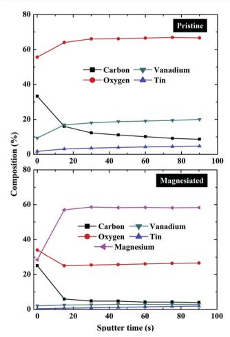
Fig. 3 XPS depth profile composition measurements of pristine and magnesiated V<sub>2</sub>O<sub>5</sub> cathodes indicating the relative contents of carbon, oxygen, vanadium, tin and magnesium as a function of overall ion bombardment time (in itself a function of depth from the surface of the sample down into the bulk).89
