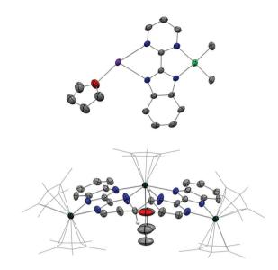
Fig. 1 ORTEP of 1(THF) (top) and 2 (bottom). Thermal ellipsoids are at 50% level. Carbon atoms are in grey, hydrogen atoms are in white and have been removed for clarity except the ones on the coupled carbons of the ligands, potassium in purple, nitrogen in blue, nickel in bright green and ytterbium atoms in deep green. Co-recrystallized solvent molecules of  $Et_2O$  in 2 are omitted. Cp\* ligands on ytterbium are presented in wireframe style for clarity.
