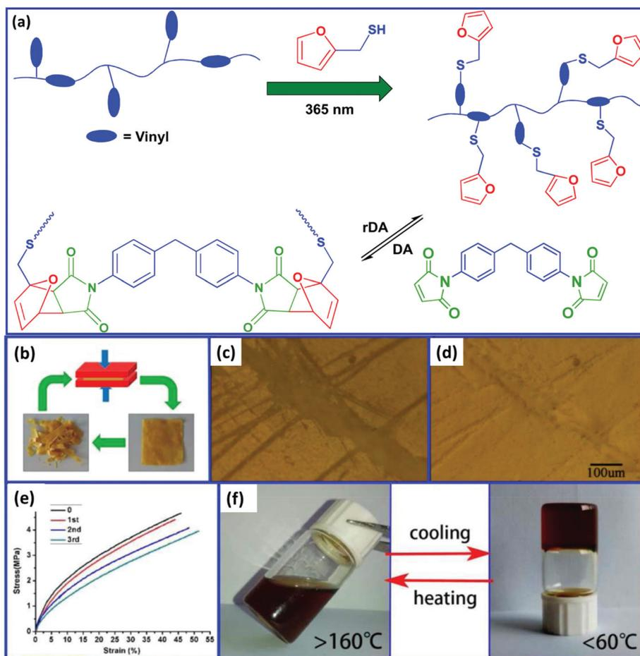
**Fig. 4** (a) Schematic representation for the preparation of the recyclable PB rubber, (b) recyclability study, (c) the photograph of the scratched film at room temperature, (d) the photograph of the film after heating at 150 °C, (e) stress–strain curves of the pristine and the recycled samples, and (f) the sol–gel process in dichlorobenzene at different temperatures.<sup>69</sup> Reproduced from ref. 69 with permission from American Chemical Society, copyright 2015.
