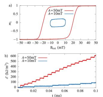
Fig. 5 (a) Hysteresis loops for an ensemble of 10 000 particles, excited with a sinusoidal externally applied magnetic field with amplitudes of 10 mT (blue lines) and 50 mT (red lines). (b) Dissipated heat by a single particle as function of time for 10 periods of the field excitation.
