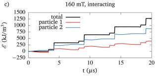
Fig. 8 (a) Hysteresis loops for particles, excited with an sinusoidal externally applied magnetic field with amplitudes of 75 mT (red lines) and 160 mT (blue lines). (b) and (c) Dissipated heat by individual particles as function of time for 10 periods of the field excitation with amplitude 75 mT [panel (b)] and 160 mT [panel (c)], respectively. These figures correspond to the cases highlighted with filled dots in Fig. 6.
