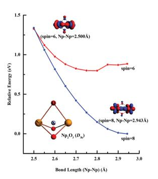
Fig. 3 Linear transit (LT) potential energy curves of  $\mathrm{Np_2O_3}$  calculated at the SR-DFT/PBE level.
