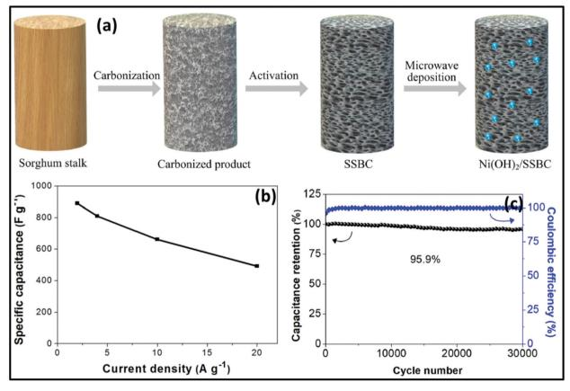
Fig. 18 (a) Synthesis of Ni(OH)<sub>2</sub>/sorghum stalk biomass carbon, (b) specific capacitance of Ni(OH)<sub>2</sub>/sorghum stalk biomass carbon composite and (c) cyclic property and columbic efficiency of Ni(OH)<sub>2</sub>/sorghum stalk biomass carbon composite. Reprinted (adapted) with permission from ref. 267, copyright (2020), Elsevier B.V. All rights reserved.
