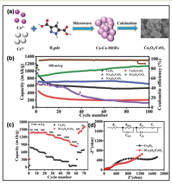
Fig. 22 (a) Schematic illustration of the preparation of  $Co_3O_4/CeO_2$ , (b) cycling performance of as-obtained samples at 100 mA  $g^{-1}$ , (c) rate performance of  $Co_3O_4$  and  $5Co_3O_4/CeO_2$ , and (d) Nyquist plots of  $Co_3O_4$  and  $5Co_3O_4/CeO_2$  after 100 cycles and the equivalent circuit diagram of the cells. <sup>319</sup> Reprinted (adapted) with permission from ref. 319, copyright (2021), Elsevier B.V. All rights reserved.
