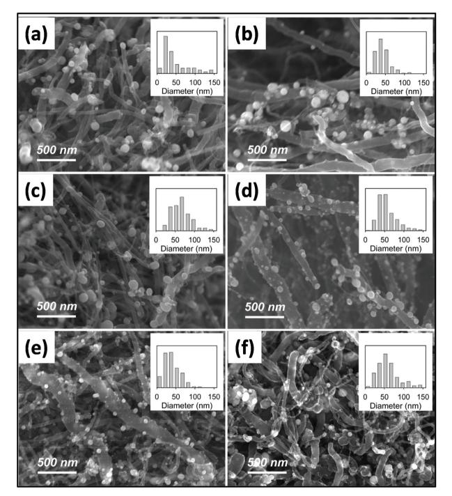
Fig. 9 SEM images of various samples of silver/MWCNT starting material (a) 1 min, (b) 2 min, (c) 5 min, (d) 10 min, (e) 30 min, and (f) 60 min, of MWI.<sup>198</sup> Reprinted (adapted) with permission from ref. 198, copyright (2011), the American Chemical Society.
