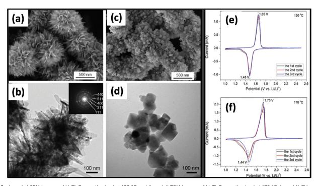
Fig. 20 (a and c) SEM images of  $Li_4Ti_5O_{12}$  synthesized at 130 °C and (b and d) TEM images of  $Li_4Ti_5O_{12}$  synthesized at 170 °C. (e and f) CV curves of  $Li_4Ti_5O_{12}$  prepared at (e) 130 °C and (f) 170 °C in the first three cycles at a scan rate of 0.2 mV s<sup>-1</sup>.<sup>281</sup> Reprinted (adapted) with permission from ref. 281, copyright (2012), Elsevier B.V. All rights reserved.
