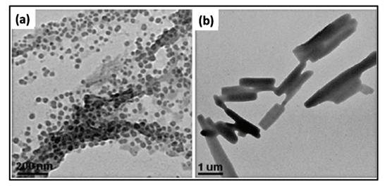
Fig. 7 TEM images of ZnO nanostructures prepared by MWI of 0.1 M zinc acetate solution in pure oleic acid for 30 s (a) and 60 s (b). 161 Reprinted (adapted) with permission from ref. 161, copyright (2013), Springer. All rights reserved.
