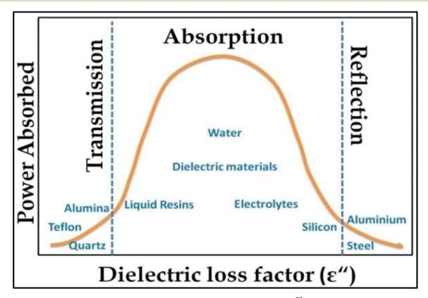
Fig. 3 Dependence of reflection, absorption and transmittance on dielectric loss factor process.<sup>97</sup> Reprinted (adapted) with permission from ref. 97, copyright (1999), Elsevier B.V. All rights reserved.
