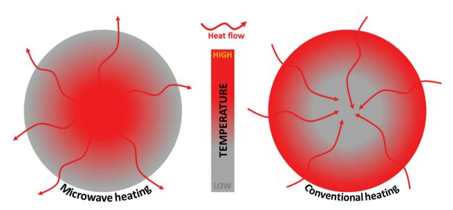
Fig. 2 Schematic representation of the temperature gradient and heat flow due to MW and conventional heating.
