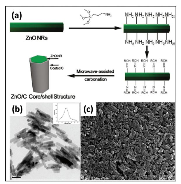
Fig. 10 (a) Schematic diagram showing the synthesis of carbon-coated ZnO. (b) TEM (inset: average size distribution of 200 rods) and (c) SEM images of ZnO nanorods.<sup>204</sup> Reprinted (adapted) with permission from ref. 204, copyright (2009), the American Chemical Society.
