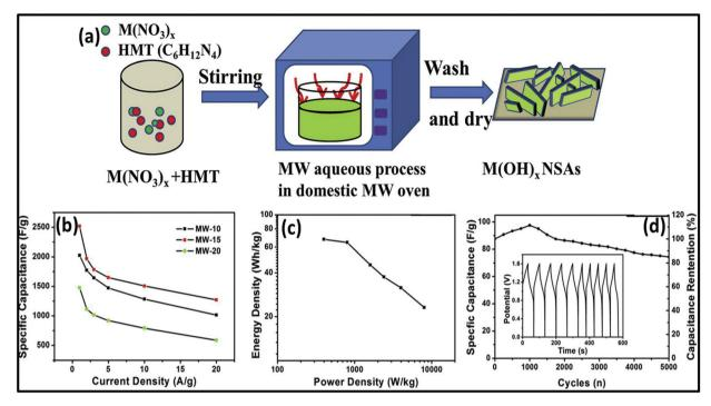
Fig. 17 (a) Schematic of MW-assisted synthesis of layered metal hydroxide nanosheet arrays, (b) specific capacitance vs. current density of  $Ni(OH)_2$  nanosheet arrays, (c) Ragone plot and (d) cycle curves of  $Ni(OH)_2$  nanosheet arrays//activated carbon aqueous hybrid supercapacitor. Reprinted (adapted) with permission from ref. 265, copyright (2019), Elsevier B.V. All rights reserved.
