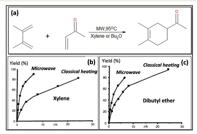
Fig. 4 (a) Schematic molecular representation and MW condition. (b) and (c) Effects of different types of heating on product yield for xylene and dibutyl ether.<sup>111</sup> Reprinted (adapted) with permission from ref. 111, copyright (1991), Elsevier B.V. All rights reserved.
