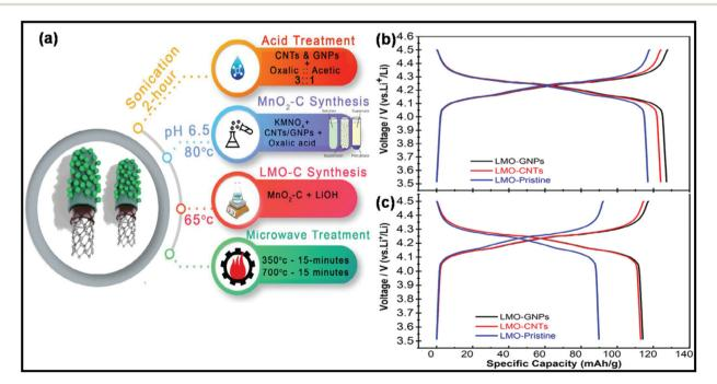
Fig. 23 (a) Schematic of the experimental details for the synthesis of LiMn<sub>2</sub>O<sub>4</sub>/CNT/GNP nanocomposite. (b) Galvanostatic charge/discharge behavior of LiMn<sub>2</sub>O<sub>4</sub>/GNPs, LiMn<sub>2</sub>O<sub>4</sub>-CNTs and pristine LiMn<sub>2</sub>O<sub>4</sub> at 0.1 C and 25 °C (b) 1st cycle and (c) 50th cycle.<sup>322</sup> Reprinted (adapted) with permission from ref. 322, copyright (2021), Wiley, All rights reserved.
