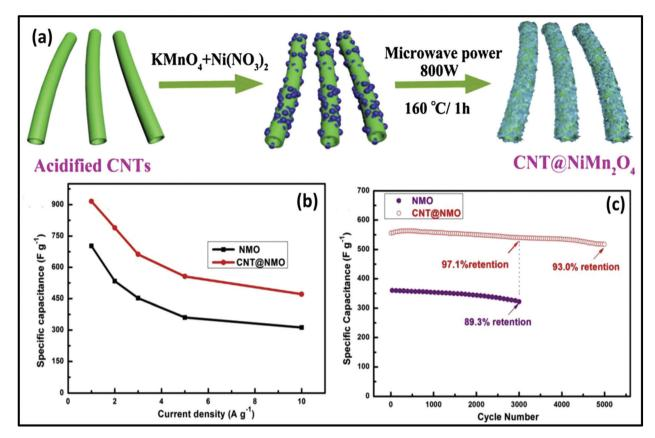
Fig. 19 (a) Schematic representation of the formation of CNT@NiMn $_2$ O $_4$  nanocomposite, (b) specific capacitance of NiMn $_2$ O $_4$  and CNT@NiMn $_2$ O $_4$  nanocomposite at different current densities and (c) cycling stability of NiMn $_2$ O $_4$  and CNT@NiMn $_2$ O $_4$  nanocomposite at 5 A g $^{-1}$ . Reprinted (adapted) with permission from ref. 273, copyright (2020), Elsevier B.V. All rights reserved.
