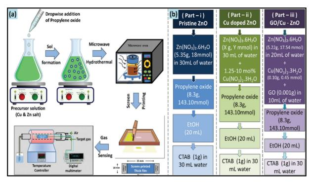
Fig. 12 Schematic illustration of the MW synthetic approach for CuO/ZnO heterojunction: (a) complete synthetic process and (b) various samples prepared in this study.<sup>219</sup> Reprinted (adapted) with permission from ref. 219, copyright (2020), the American Chemical Society.
