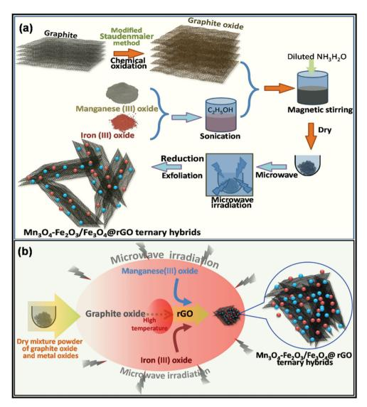
Fig. 13 Schematic presentation of the (a) synthesis process and (b) mechanism of MW-assisted formation of Mn<sub>3</sub>O<sub>4</sub>-Fe<sub>2</sub>O<sub>4</sub>@rGO ternary hybrid.<sup>222</sup> Reprinted (adapted) with permission from ref. 222, copyright (2020), Elsevier B.V. All rights reserved.
