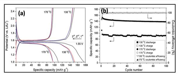
Fig. 21 (a) Galvanostatic charge/discharge curves for  $\text{Li}_4\text{Ti}_5\text{O}_{12}$  prepared at 130 °C and 170 °C between 1 and 2.5 V at a current density of 200 mA  $\text{g}^{-1}$ . (b) Cycling performance of  $\text{Li}_4\text{Ti}_5\text{O}_{12}$  prepared at 130 °C and 170 °C measured at a current density of 200 mA  $\text{g}^{-1}$ . Reprinted (adapted) with permission from ref. 281, copyright (2012), Elsevier B.V. All rights reserved.
