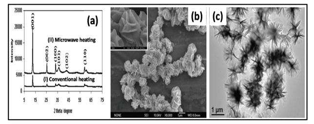
Fig. 8 (a) XRD pattern of  $\alpha$ -Ni(OH)<sub>2</sub> synthesized by (i) conventional heating method and (ii) MW heating method. (b) SEM image of  $\alpha$ -Ni(OH)<sub>2</sub> and (c) TEM image of α-Ni(OH)<sub>2</sub>.<sup>179</sup> Reprinted (adapted) with permission from ref. 178 and 179, copyright (2008 and 2010), the American Chemical
