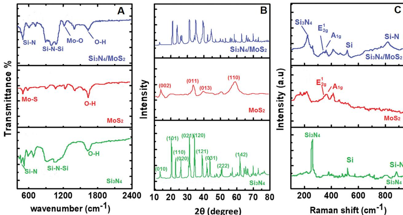
Fig. 1 (A) FTIR spectra, (B) XRD patterns, and (C) Raman spectra of Si<sub>3</sub>N<sub>4</sub>, MoS<sub>2</sub> and the Si<sub>3</sub>N<sub>4</sub>/MoS<sub>2</sub> composite.
