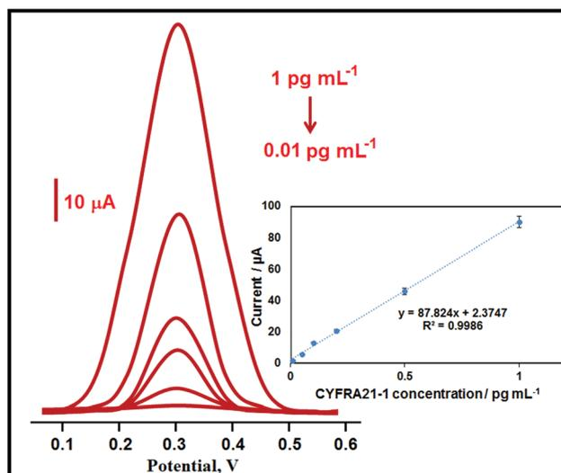
Fig. 4 Concentration effect (from 0.01 to 1.0 pg mL<sup>-1</sup> CYFRA21-1) on immunosensor signals, inset: the calibration curve for the voltammetric CYFRA21-1 immunosensor.
