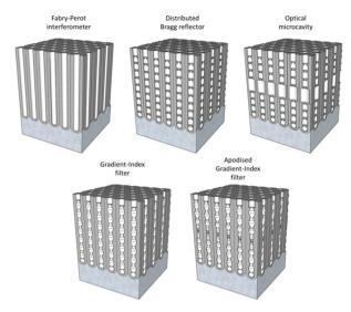
**Fig. 23** Structural details of the photonic crystal structures made from nanoporous AAO membranes by structural engineering of the effective medium.
