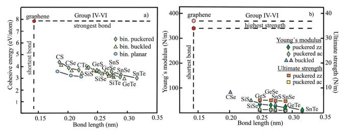
Fig. 21 (a) Cohesive energy *versus* bond lengths of binary group IV–VI monolayers. (b) Young's moduli and ultimate strengths *versus* bond length of binary group IV–VI monolayers.
