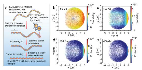
Fig. 4 (a) Schematic illustration for the orientation process of a flexible PNC under H. (b-e) The calculated probabilities of different conformations shown by 50 000 flexible PNCs under different H values.
