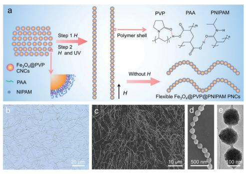
Fig. 1 The preparation and characterization of the typical  $Fe_3O_4$ @PVP@PNIPAM flexible PNCs. (a) Schematic illustration showing the formation process of the  $Fe_3O_4$ @PVP@PNIPAM flexible PNCs; (b) bright-field optical microscopy image; (c and d) SEM images; (e) TEM image.
