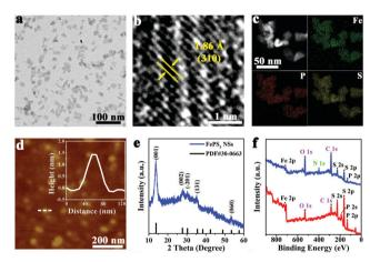
Fig. 1 (a) TEM image, (b) HRTEM image, (c) HAADF-STEM image and the corresponding EDS elemental mapping images, (d) AFM image with height profile, and (e) XRD pattern of FePS<sub>3</sub> NSs. (f) XPS survey spectra of FePS<sub>3</sub> NSs (blue) and bulk FePS<sub>3</sub> (red).
