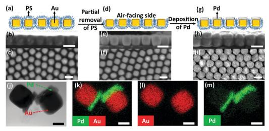
Fig. 1 Fabrication of Janus plasmene nanosheets. (a, d, and g) Scheme of fabricating Janus plasmene nanosheets. Cross-section SEM image of (b) PS-capped, (e) one-side exposed and (h) Janus plasmene nanosheets on a Si wafer and (c, f, and i) their corresponding top-view SEM images. (j) Dark-field TEM images of individual Janus NPs and (k-m) corresponding EDX elemental mapping images (red: Au; green: Pd). (Scale bar: 50 nm for SEM, 20 nm for TEM.)
