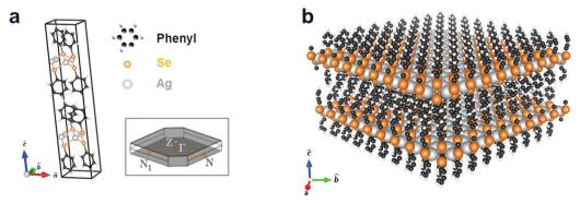
Fig. 1 Silver benzeneselenolate ([AgSePh] $_{\infty}$ ) unit cell and molecular structure. (a) Primitive cell and first Brillouin zone (inset); see ESI $_{\uparrow}$  for cell coordinates. (b) Extended layered molecular structure of [AgSePh]<sub>∞</sub> consisting of 2D sheets of AgSe spaced by phenyl groups.
