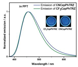
Fig. 4 Photoluminescence spectra of  $CF_3CzpPhTRZ$  and CNCzpPhTRZ dispersed at 10 wt% in PPT matrix at 295 K ( $\lambda_{exc}$  = 360 nm).
