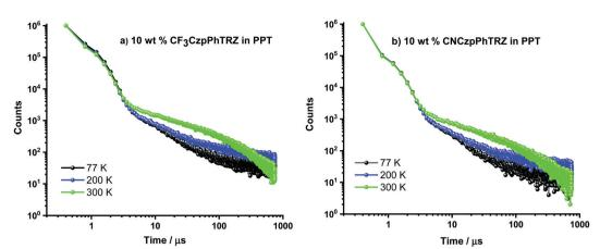
Fig. 5 Temperature-dependent time-resolved photoluminescence lifetime of 10 wt% doped films of (a) CF<sub>x</sub>CzpPhTRZ and (b) CNCzpPhTRZ in PPT  $(\lambda_{exc} = 379 \text{ nm}).$
