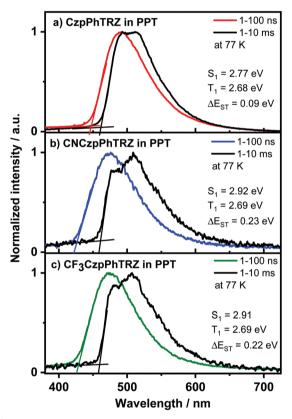
Fig. 6 77 K prompt PL and phosphorescence spectra measurement of 10 wt% (a) CzpPhTRZ (b) CF3CzpPhTRZ and (c) CNCzpPhTRZ doped in PPT host ( $\lambda_{\rm exc}$  = 343 nm), the  $\Delta E_{\rm ST}$  value is taken from the onset value difference between the 77 K prompt fluorescence and phosphorescence spectra.
