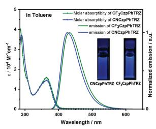
Fig. 3 Molar absorptivity and photoluminescence spectra of  $\mathbf{CF_3CzpPhTRZ}$  and  $\mathbf{CNCzpPhTRZ}$  in toluene at 298 K ( $\lambda_{\mathsf{exc}}$  = 360 nm). Inset: photos of photoexcited solutions in toluene.
