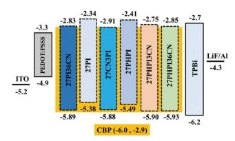
Fig. 6 Energy-level diagrams of the materials used in the fabrication of the OLED devices
