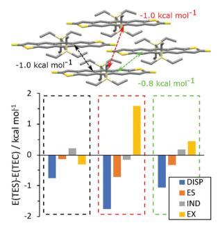
Fig. 5 Difference in SAPTO interaction energies (E(TES) min E(TEC)) for relaxed 2D packing structures.
