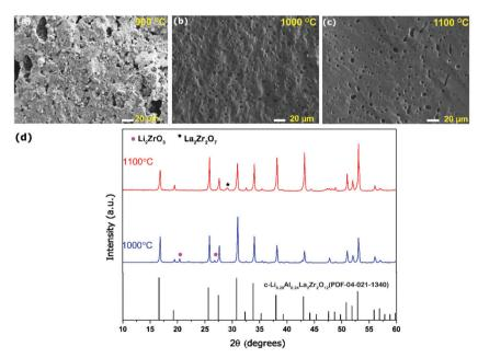
Fig. 5 SEM fractured surface images of Al-LLZO pellets sintered at (a) 900 °C, (b) 1000 °C, and (c) 1100 °C, and (d) XRD patterns of the conductive pellets sintered at 1000 °C and 1100 °C for 6 h (c-Li<sub>6.28</sub>Al<sub>0.24</sub>La<sub>3</sub>Zr<sub>2</sub>O<sub>12</sub> phase # PDF: 04-021-1340, Li<sub>2</sub>ZrO<sub>3</sub> phase PDF # 016-0263 and La<sub>2</sub>Zr<sub>2</sub>O<sub>7</sub> phase # 01-070-5602).
