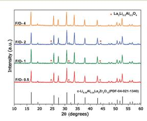
Fig. 2 XRD patterns of calcined Al-LLZO samples with various fuel to oxidizer (F/O) ratios.
