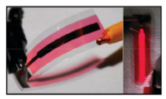
Fig. 17 Image of slot-die coated flexible OLEDs (left) without bias voltage (right) red light emission with bias voltage (reprinted with the permission from the ref. 42)
