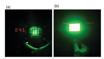
Fig. 13 Emission of green light from (a) small area (2 mm  $\times$  2 mm) and (b) large area (43 mm  $\times$  29 mm) slot-die coated OLEDs (reproduced with permission from the ref. 94).
