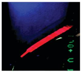
Fig. 9 Image of a flexible OLED with slot-die coated HTL (PEDOT:PSS) and EML (F8:tPDI<sub>2</sub>N-EH) under operation and emitting red light (taken from the ref. 91).
