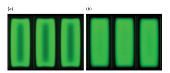
Fig. 20 Image of light emission from the OLEDs pixel (75  $\times$  180  $\mu$ m) where slot-die coated PVK annealed under (a) atmospheric pressure and (b) partial vacuum (reprinted with permission from the ref. 102).
