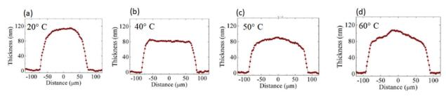
Fig. 22 Thickness profile of PEDOT:PSS stripe coated at pre-drying temperatures (a) 20 °C (b) 40 °C (c) 50 °C and (d) 60 °C (reprinted with the permission from ref. 107).
