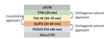
Fig. 16 Schematic of OLEDs structure with four organic layers. QUPD is N,N-bis(4-(6-((3-ethyloxetan-3-yl)methoxy)hexyloxy)phenyl)-N,N-bis(4methoxyphenyl)biphenyl-4,4-diamine, TSG-M is green emitter. (reproduced from the ref. 95).
