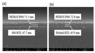
Fig. 7 SEM image of HTL/PEDOT:PSS interface (a) small molecule HTL (b) hybrid HTL (reprinted with the permission from the ref. 89).
