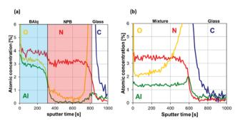
Fig. 25 XPS profile of NPB and BAlq bilayer (a) when BAlq coated with orthogonal solvent and (b) when BAlq coated from non-orthogonal solvent (reprinted with permission from ref. 110).
