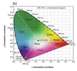
Fig. 4 (a) Equations to calculate the color space coordinates, (b) Chromaticity diagram CIE 1931 in 2-dimension plane (reprinted with permission from the ref. 70)
