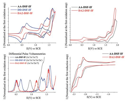
Fig. 1 Electrochemical studies of **AA-DSF-IF** (black), **DD-DSF-IF** (blue) and **DA2-DSF-IF** (red). Cyclic voltammetries recorded in  $Bu_4NPF_6$  0.2 M in  $CH_2Cl_2$  (top) and in THF (bottom right). Working platinum disk electrode. Sweep-rate 100 mV s<sup>-1</sup>. Differential pulse voltammetry recorded in  $Bu_4NPF_6$  0.2 M in  $CH_2Cl_2$  (Bottom Left). Working platinum disk electrode. Pulse height: 50 mV, Scan-rate: 10 mV s<sup>-1</sup>.
