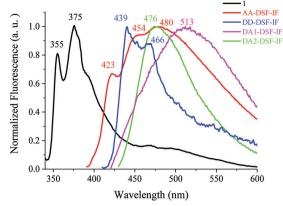
Fig. 4 Emission spectra in cyclohexane (left) and in the thin film (right) of 1 ( $\lambda_{\rm exc}$  = 310 nm, black), AA-DSF-IF, DD-DSF-IF, DA1-DSF-IF and DA2-DSF-IF,  $\lambda_{\rm exc}$  = 350 nm.
