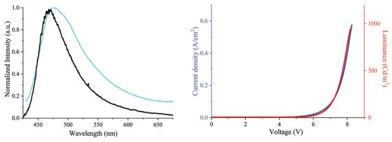
Fig. 8 Left: EL spectrum of the DA2-DSF-IF-based device (black line) and the PL spectrum of the DA2-DSF-IF thin film (cyan line). Right, IVL characteristic (luminance: red line, current density: blue line).
