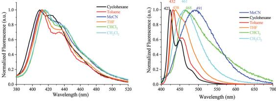
Fig. 6 Emission spectra of AA-DSF-IF ( $\lambda_{\rm exc}$  = 300 nm) and DD-DSF-IF ( $\lambda_{\rm exc}$  = 390 nm) in different solvents.
