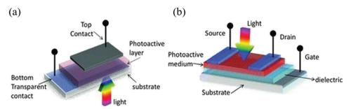
Fig. 7 The schematic diagram of device configurations of (a) the vertical structure and (b) the lateral structure (Reproduced from ref. 104 with permission from 2013 Wiley-VCH).
