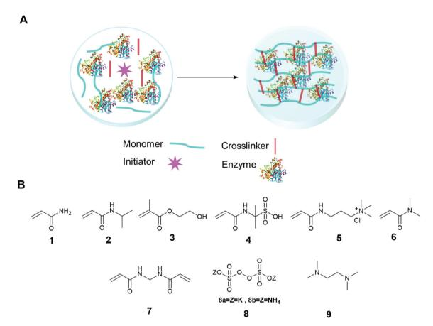
Fig. 7 Enzyme entrapment in synthetic polymer gels. (A) Schematic presentation of entrapment in synthetic polymer gels; (B) chemical structure of some common monomers, crosslinker and initiators.
