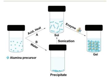
Fig. 6 Different approaches (A and B) to entrapping enzymes in alumina (boehmite) gels by sol-gel methods.
